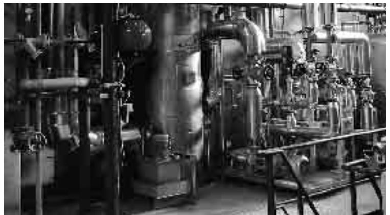
Transformer drying plant with rotary vane pumps UnoLine™
