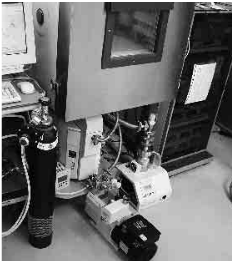
Turbopumping station TSU 071 Economy for CO 2 gas analysis
