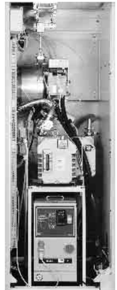
Coating unit with rotary vane pump DUO 35 and a turbopump TPH 2101
