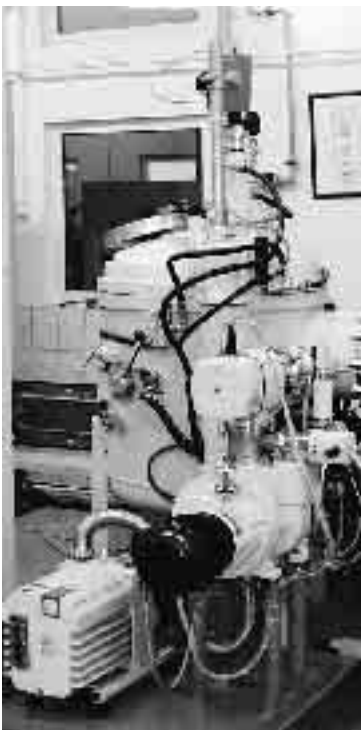
Pumping station with Roots pump and rotary vane pump DUO 65 M
