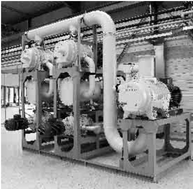
Roots pumping station for removing zinc from molten steel
